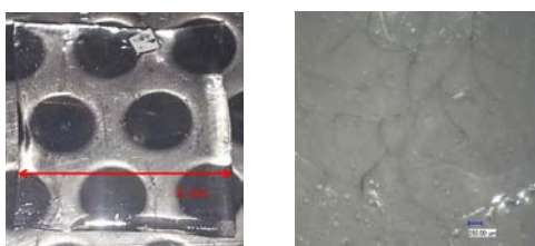
Figure 1: Left: EVA sample 1 became semifluid and tenacious after 117 kWh/m 2 at 60 °C. Right: After 312 kWh/m 2 the sample hardened and cracks are visible.
